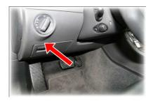
When the navigation has booted, connect the CTVIMAU03 interface to the OBD-socket for about 15 seconds in order to activate the function. Disconnect the CTVIMAU03 from the OBD-socket.
