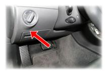
When the navigation has booted, connect the CTVIMAU02 interface to the OBD-socket for about 15 seconds in order to activate the function. Disconnect the CTVIMAU02 from the OBD-socket.
