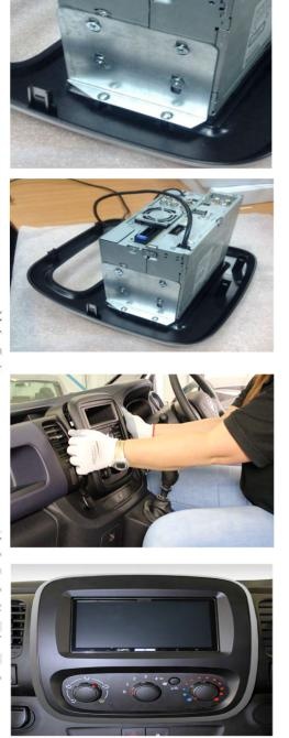
5. Attach the brackets to the Radio and Fascia
