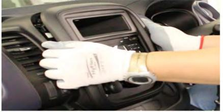
2. Once the panel is removed please extract the screws and the Radio as shown on the image below
