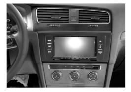
Connect all cables, insert the unit into the housing and verify the proper functioning of the system. Take the supplied facia plate, place on it the silver frame and the air vents and mount the assembly on the dashboard.
