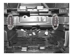
Cut and remove the plastic "bridge" at the points indicated by the white dotted lines.
