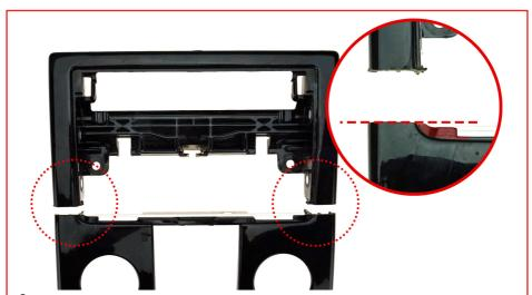
**2.** The original panel will need to be cut. See highlighted section. Cut the centre panel in line with the highlighted tab just above the bottom of the opening on each side. The aftermarket fascia panel will cover the cut marks however please do this as straight and neat as possible.
