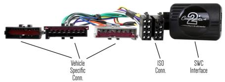
Connect the 12 Pin black connector of the stereo patch lead to the interface.
