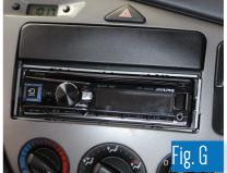
Surround the stereo with the trim panel (included with the new stereo) to complete the installation (Fig. H).
