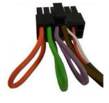
NB: When cutting loops on the CTMULTILEAD.2, please ensure that the bare wire ends are insulated
