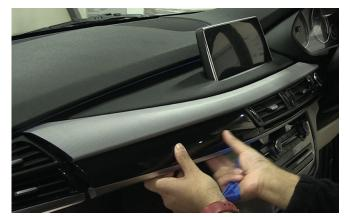
Still using the panel removal tool, begin to lever off the air vent panelling. Ensure to do this carefully so not to break any clips or damage the surface. Once free, remove whilst disconnecting the hazard switch and stop/start connectors.
