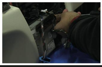
With the main fascia panel out of the way, proceed to undo the 4x screws that hold the main head unit in place. Once free, pull out and disconnect all of the wiring.
