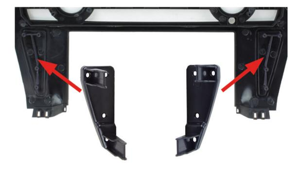
Take the 2x fascia locater brackets within the kit and line them up to the appropriate side of the fascia as indicated by the plastic grooves. Once lined up correctly, use the 8x self taping screws to attach them to the back of the fascia.
