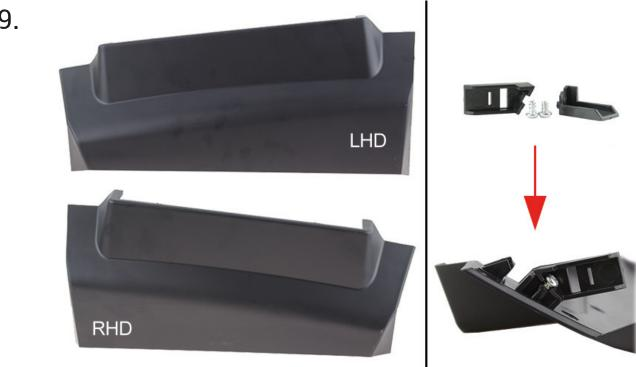
Select one of the bottom trim panels dependent on the orientation of the vehicle. Once selected, take the 2x locater clips found within the kit and attach them in the location seen here with the 2x screws provided. When fully attached, transplant the 2x OEM metal clips from the original bottom panel onto these locater clips.
