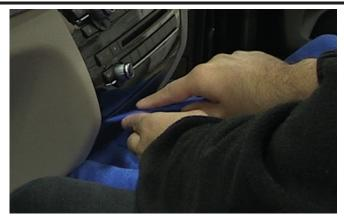
Begin by using a panel removal tool to remove the bottom trim panel.
