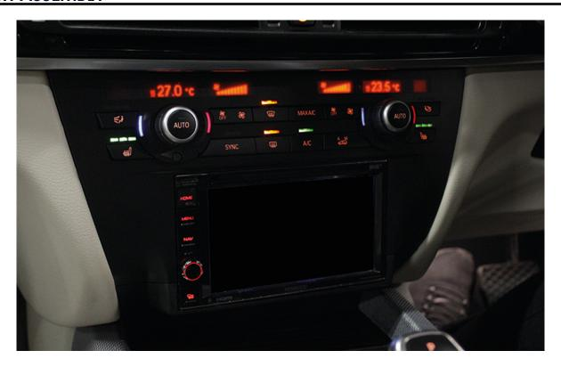
Reassemble the rest of the dashboard to complete the installation. When installed the vehicles original LED display will now be viewable alongside your new installed stereo.
