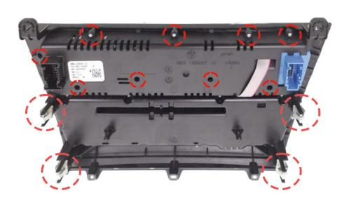
Take the original fascia and remove the 4x screws along the top, as well as the 5x recessed screws (shown in image) holding the top climate control button panel in place. You will also need to remove the 4x metal clips highlighted.
