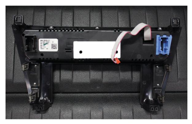
Take the new fascia and transplant the top climate control button panel into the opening, securing it in place using the 9x pre-existing screws removed in step 7. In addition, fix the 4x metal clips onto the new locator posts again removed in step 7.
