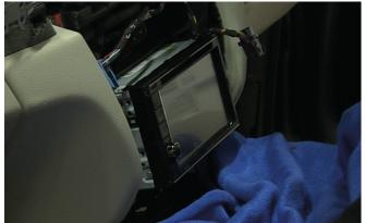
With the brackets affixed to the correct sides of the stereo, connect up the stereo and slot into place, screwing into place using the 4x pre-existing screws.
