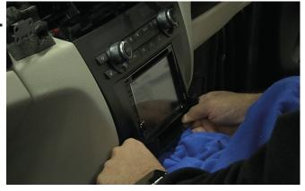
Take the bottom trim panel and slide it underneath the new stereo using the clip locaters as guides to firmly clip it into place.
