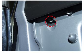
Now open the glovebox, within the lip on the far side nearest to the passenger side door will be a recessed torx screw. Once this screw has been undone, proceed to fully remove the dashboard trim by means of a panel removal tool, disconnecting the button panel in the process.
