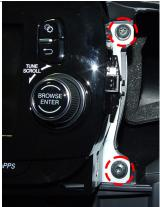
When the main fascia trim has been removed, undo the 4x screws found on either side of the main unit and proceed to pull it out of the dash whilst disconnecting all of the wiring.
