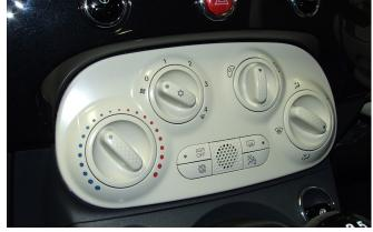
To begin, use a panel removal tool to unclip the climate control button panel. Be careful not to damage the surrounding trim.
