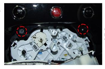
Once the climate control button panel is out of the way, proceed to undo the 2x torx screws located at the top of the aperture.
