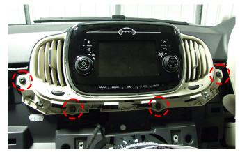
With the dashboard trim panel out of the way, proceed to undo the 4x highlighted torx screws that surround the main fascia trim. Once free, pull upwards away from the dash.
