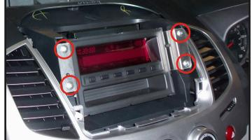
With the trim removed, undo the 4x screws that surround the trip computer and remove it whilst disconnecting all of the wiring.
