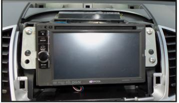
With the brackets correctly aligned (and the stereo wired up) screw the new stereo into place using the pre-existing screws.
