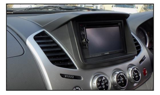
Finally, place the new hood fascia panel over top the new stereo and fix into place using the clips provided.
