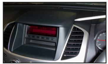
Begin by using a panel removal tool to pry the main fascia hood trim up and away from the dashboard.
