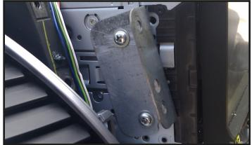
Attach the brackets to both sides of the stereo and fit loosely into the dashboard to gauge the correct orientation.
