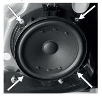
Use a 4mm drill to remove the rivets. Make sure all remains from the old rivets are removed from the inside of the door.
