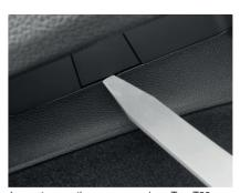
In most cases the screws used are Torx T30. Unscrew them and store them in a safe place, to re-use when re-mounting the door panel.
