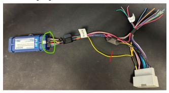
STEP 3 –Route the wire from the RP4-CH11 harness to the accessory port. The image below shows the routing for a Jeep Wrangler for reference.
